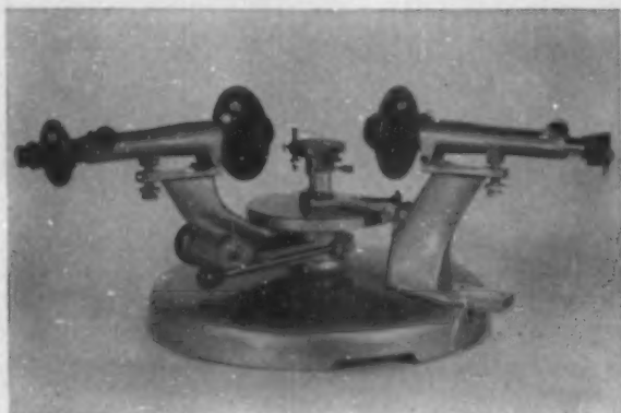
L111P Polarizing Assembly on L114 Divided Circle Spectrometer
